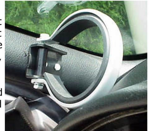
Once the base is installed, slide the tach into the mounting ring and mark the spot under the rear of tach where the hole will be drilled to pass the wires through the dash. Do not drill yet.
