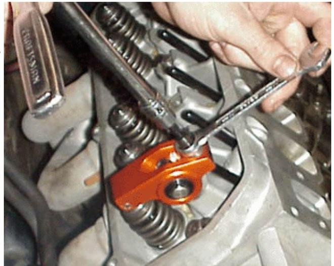
Set the desired preload with the adjuster and lock down the locknut. Now, go to the exhaust valve and repeat the process. After #1 intake and exhaust valves are complete, move to the next cylinder and repeat the process, until all 6 cylinders are complete.
