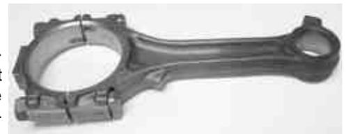
prepped rods will be able to go past 350 horsepower with no problem. Our forged pistons are designed to work with the stock forged rods with press-fit pins except we'll include lighter weight thinner wall pins.
