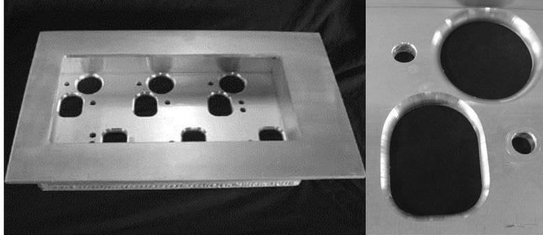
**M-112 Supercharger Adapter:** This adapter mounts directly to the lower intake manifold and is designed for use of the 03-04 Cobra M-112 supercharger on your V6. Fabricated from high strength aluminum alloy and TIG welded, includes generously radiused CNC port openings for perfect port entrance. This intake is now available 1" shorter in height to improve hood clearance, use of a raised cowl hood may be required. Includes handy installation instructions. **\$950**
